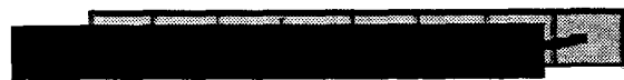
Fig. 4. Translation convergence. The prototype, shown in light gray, almost overlays the image which is shown in dark gray. Each image consists of 8 pixels in a line. The prototype is offset from the test image by 1 pixel.
