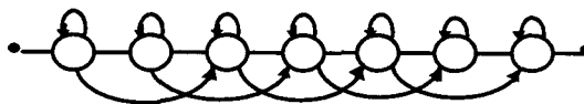
Fig. 3: Hidden Markov model (HMM) for characters. Shown is a 7-state model. For OCR, we have used 14-state models.
