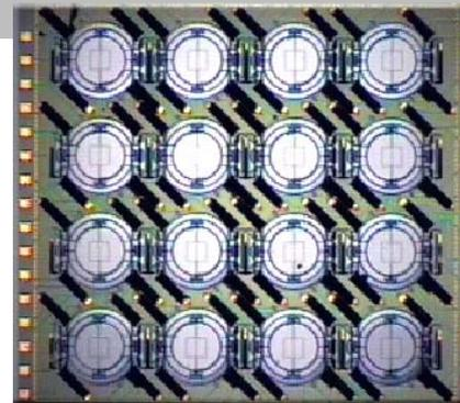
4x4 array of 2-axis micromirrors
