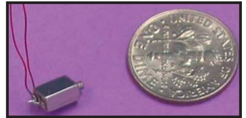
Tiny speakers are used to measure HRTF.
